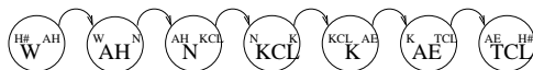
Figure 10.11: A network of triphone models representing the phrase “one cat.” Phones are written in the TIMIT transcription system ([Zue et al., 1990]).
