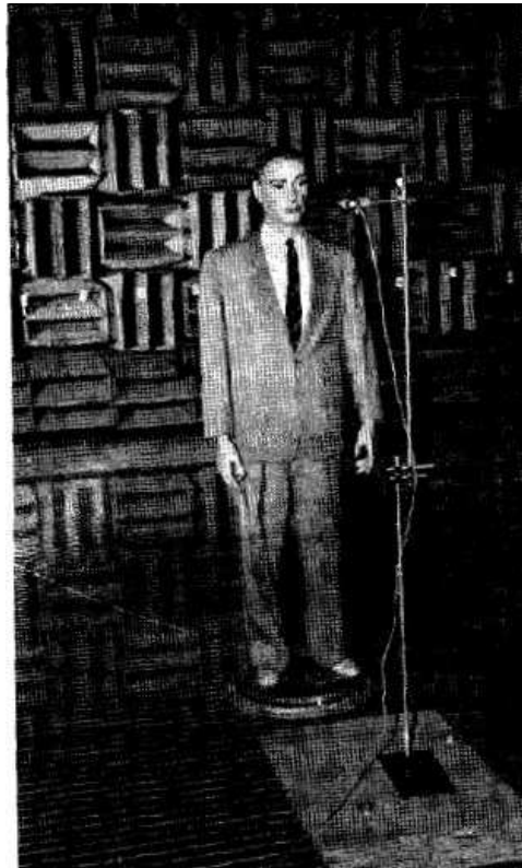
Figure 4.4: Life-size mannequin for measuring the relation between the mouth volume velocity and the sound pressure at an external point. The transducer is mounted in the mannequin's head.
